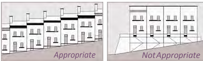
Appropriate mass grading of a site allows narrow footprint buildings to step up and follow the site topography.
